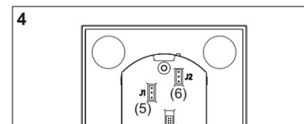
To activate the LEDs via the connected system, the corresponding jumper (Figure 4) on the back of the glass sensor must be adjusted.
